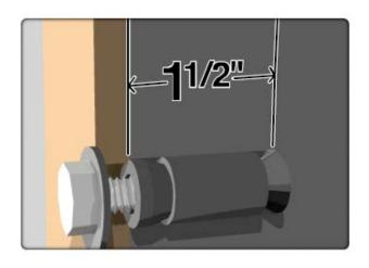
For windows 3 feet by 4 feet or smaller installed on a <u>masonry house</u>, use 1/4 inch expansion bolts and galvanized permanent expansion anchors.
