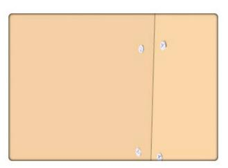
Attach the 2X4s to the <u>outside</u> of the plywood panel with 10 gauge, 2 inch long galvanized screws (exterior deck screws) spaced every 4 inches.
