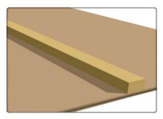
If a window or door is larger than a sheet of plywood, you will need to join the panels with 2X4 bracing along the entire seam.
