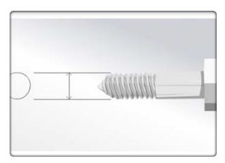
First drill holes in the same diameter as the bolts or screws, 2-inches in from the edges of the plywood at each corner and at 12inch intervals around the panel.
